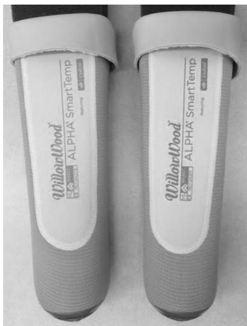
Figure 1. A SmartTemp liner and a placebo liner worn by one of the subjects with a transtibial amputation.
