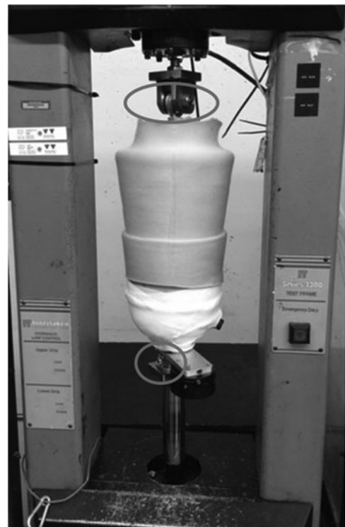
Figure 1. The tension–compression testing platform used in the study. Circles indicate the connection points of the socket and residual limb model to the tension–compression machine.
